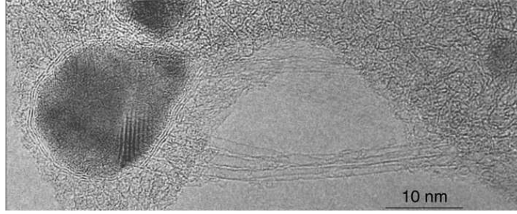
Fig. 34. HRTEM images illustrating the link between the carbide at the particle surface and the roots of the long ropes. The carbide platelet is lying at the top of the particle and seen with a fringe contrast, adapted from [204]
