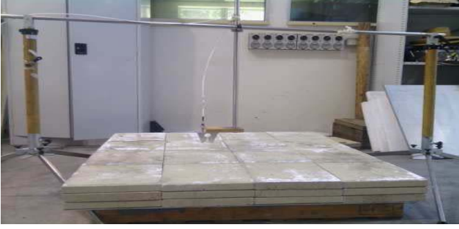
Fig. 12. Experimental setup in the case of a lossy ground, showed with a stack of three clay pavers (the results presented in this paper use a thickness of seven pavers).
