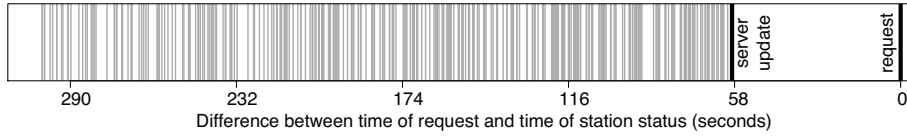
Figure B.1: This example shows difference in time between the request, server update of station states file (60 seconds) and individual station states (mean of 150 seconds).
