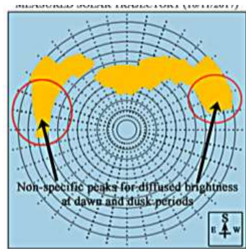
Fig. 2 - Solar trajectory through assessing brightest sky-positions
