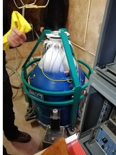
Figure 2.8: (a) Concept sketch of the core element of the superconducting gravimeter, that is the part inside the liquid Helium with the gravity sensing element. From Goodkind (1999). (b) Superconducting gravimeter of the Royal Observatory of Belgium in the underground Membach station during a Helium refill. Picture taken by the author.
