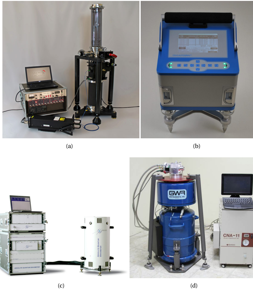
Figure 2.12: Overview of commercial gravimeters. (a) FG5-X. From http://microglacoste.com/product/fg5-x-absolute-gravimeter/ . (b) CG-6 Autograv. From https://scintrexltd.com/product/cg-6-autograv-gravity-meter/ . (c) Absolute Quantum Gravimeter. Form https://www.muquans.com/product/absolute-quantum-gravimeter/ . (d) iGRAV Gravity Sensors. From https://www.gwrinstruments.com/igrav-gravity-sensors.html . All accessed on 14.02.2022.
