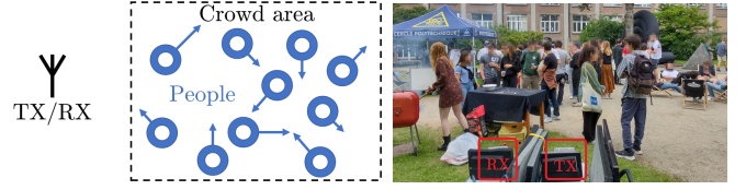
Fig. 2. Crowd counting scenario (left) and measurements scene (right), with TX and RX seen from behind.
