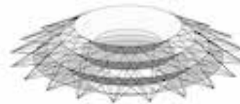
D. Bracing cables
