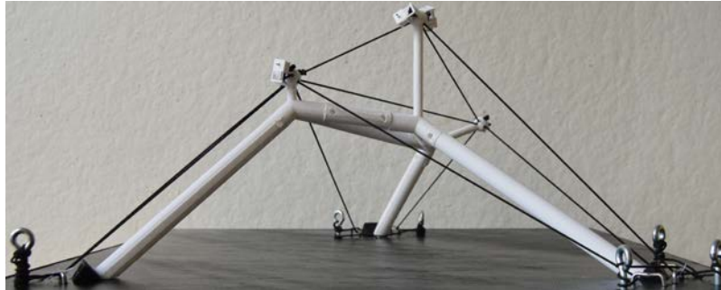
Figure 12: Reduced-scale model of an externally post-tensioned spatial funicular structure.
