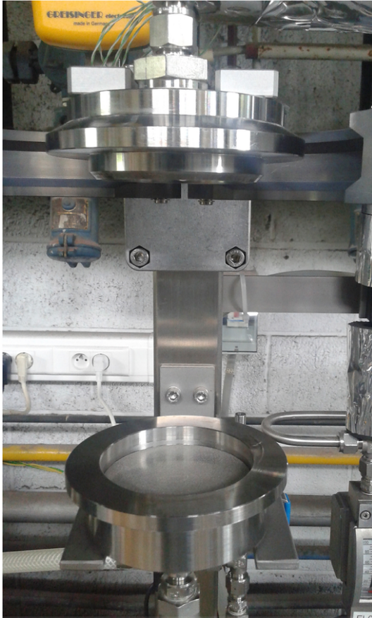
Fig. 2. The cell for preparing supported ionic liquid membrane.
