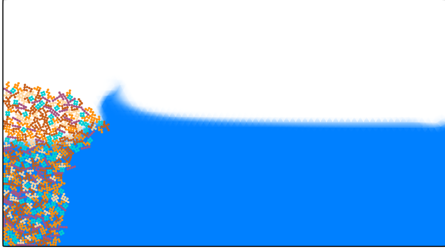
Fig. 5.4: Snapshot of the simulation of the two-dimensional collapse of a partially submerged column made of grains with shapes inspired from the Tetris game. The grains are coloured according to their moment of inertia. The fluid is coloured according to the corresponding phase: blue for water, white for air.
