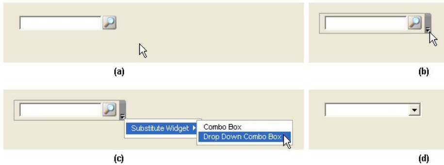
Fig. 6. Sequence of user actions to trigger a beautification operation: (a) selection, (b) contextual menu, (c) selecting a beautification operation, (d) applying it.
