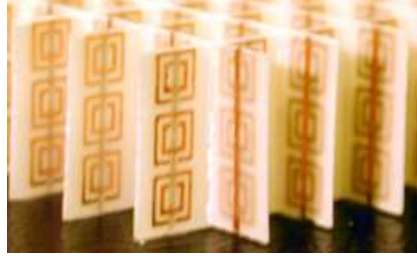
Figure 1.6: The double negative metamaterial used in the experimental verification at the University of California.
