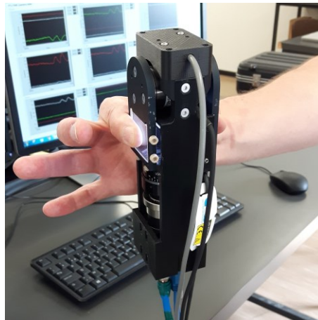
Fig. 4.2. Subject holding the manipulandum in precision grip during experiment. A transparent plate and a custom optical system allows imaging of the fingertip contact for one of the two fingers pressed against the object.
