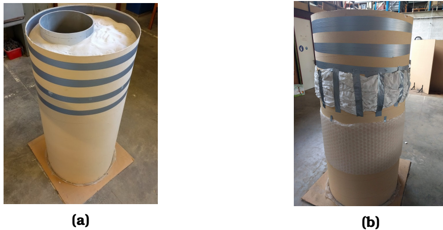
Figure 4: Laboratory tree trunk model: a) with a smooth surface, b) with a bark.
