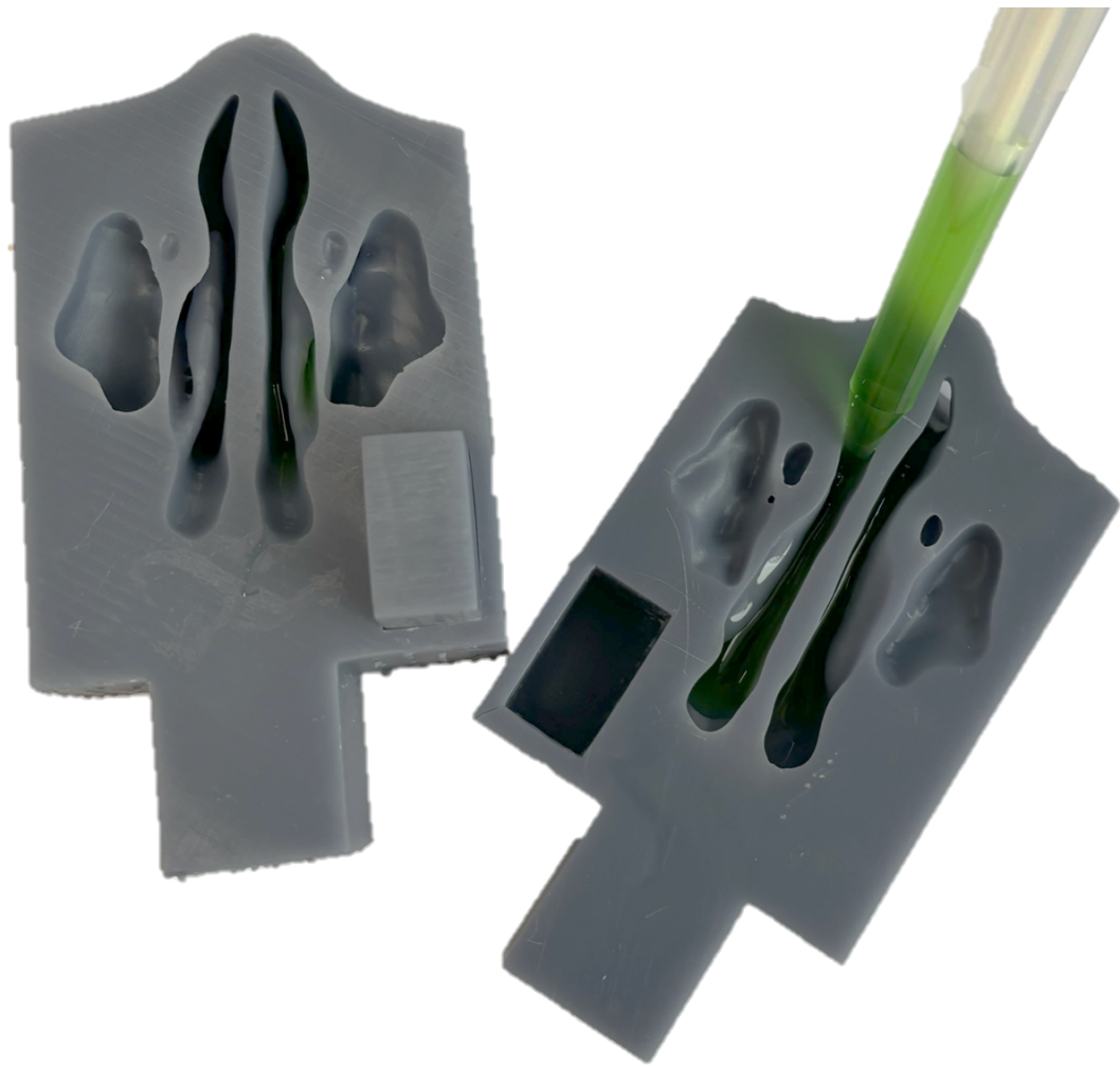
Figure 2: Hydrogel insertion in the nasal cavities of the upper airway model
