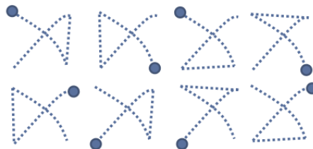
Figure 2.26 The 8 unistroke permutations for a two-stroke x based on the two-stroke gestures in Figure 2.25.
