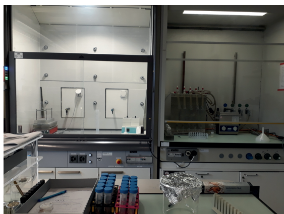
Fig. 1: A new hood (on the left) for preparation of cellulose samples; the Soxhlet system and solvents are located in the hood on the right.
