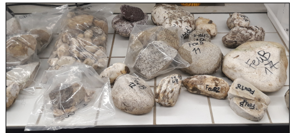
Fig. 2: Collection of quartz-rich clasts from the lowermost gravel layer of Feusi further processed for the isochron-burial dating with ^{26}\text{Al} and ^{10}\text{Be} .
