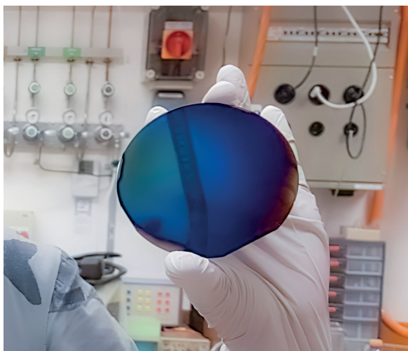
Fig. 1: BTO film grown on a Si wafer by HV-CVD.
