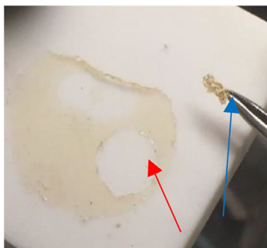
FIGURE 3 | Sample cast on a PTFE plate from which a disk was cut (red arrow). After peeling the disk off the PTFE plate, the obtained membrane shrank and was stuck onto itself, leading to an unusable sample (blue arrow).
