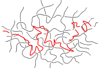
Figure 1.9: A single polymeric chain in its environment. Adapted from [17].
