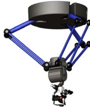
FIGURE 4.2 – SurgiScope (ISIS), porte-microscope à architecture Delta
