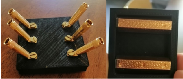
Figure 4.20. | Configuration for measuring surface resistivity using parallel electrodes.
