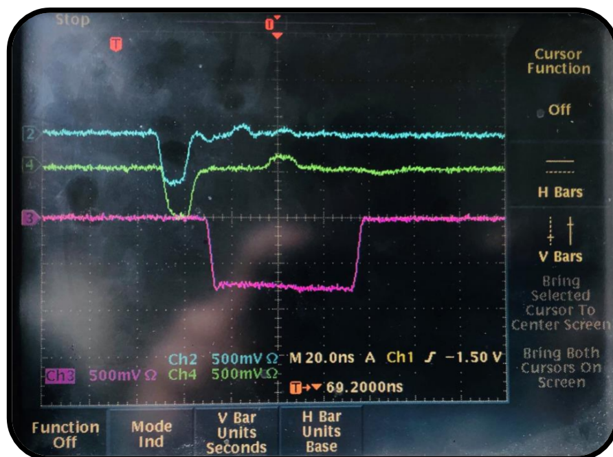
Figure 4.10. | The coincidence signal (shown in pink) within a 70 ns window, with two digitized signals from PMT A (shown in blue) and PMT B (shown in green).
