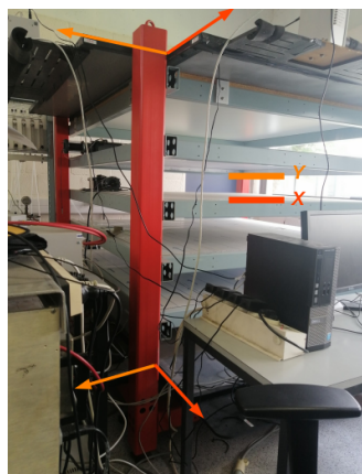
Figure 2.10. | The actual setup of the cosmic bench in our laboratory, including the frame of reference.
