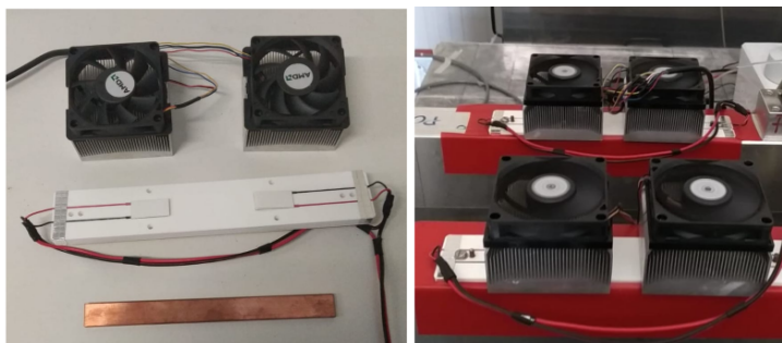
Figure 3.7. | The temperature control system. Left: the elements before installing on the detector. Right: the system installed on the detector.
