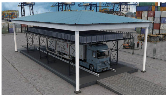
Figure 1.8. | Large area detectors of Decision Sciences for the scanning of commercial trucks. Reproduced from [57].
