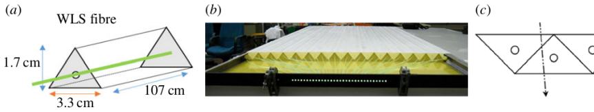
Figure 3.4. | (a) The scintillator bars possess a triangular form and are coated with a white oxide layer. Each scintillator houses a wavelength-shifting (WLS) fiber running through its center. (b) These 32 bars are bonded together in a half-plane section approximately 50 cm wide. (c) A center-of-mass algorithm is employed to reconstruct the muon coordinate based on the light collected by two adjacent scintillators.
