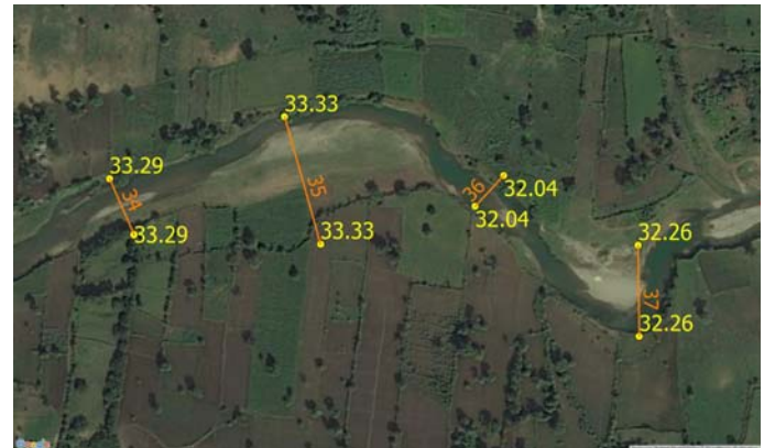
Figure 10: Example of fixed levels (in yellow) for spline interpolation – Q = 535 \text{ m}^3/\text{s} , n = 0.030 – Section 34 corresponds to PK7.062 and section 37 to PK7.720
