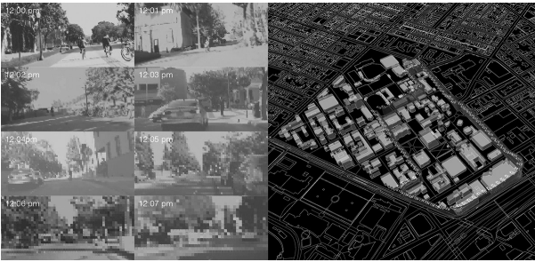
Figure 7 a) Bicycle mounted sensor kit + camera on the University of Southern California campus. Image processing based on dynamic data collected using bicycle (pixel color: temperature variation, pixel scale: ppm concentration variation); b) Aerial view of collected Data (line color: temperature variation, line scale: CO 2 variation).
