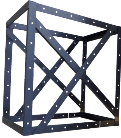
Fig. 1 Calibration cube used in swimming pool to create the calibration matrix on MatLab. Cube from SeaGIS EventMeasure.
