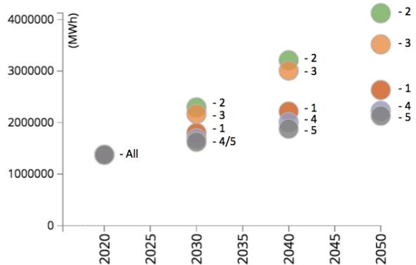
Figure 6: Evolution of total embodied energy of materials used to retrofit the dwellings in BCR for the five scenarios.
