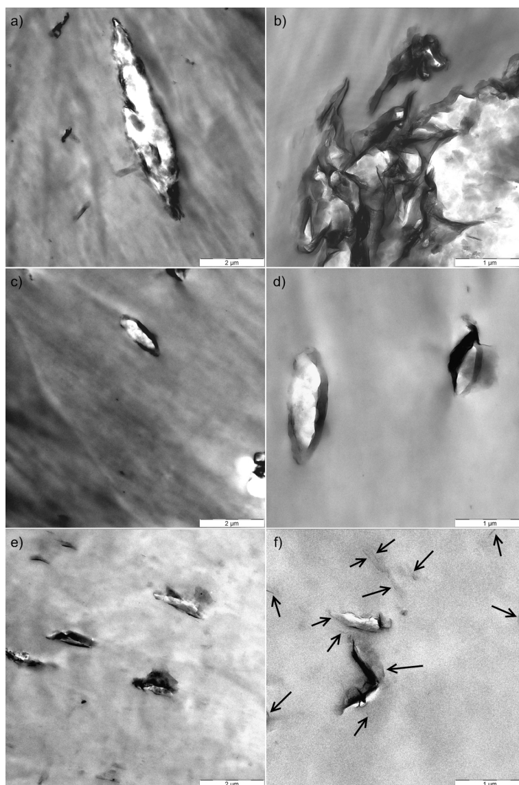
Figure 5.10: TEM pictures of NC-OP0 (a,b), NC-OP1 (c,d) and NC-OP2 (e,f) at a magnification of 2,300 and 5,000 respectively. Exfoliated clay layers are indicated with arrows.
