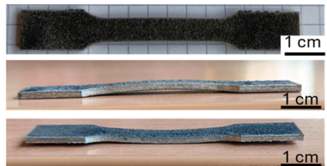
Fig. 5. Distortion of a tensile specimen observed after a heat treatment at 580 °C.
