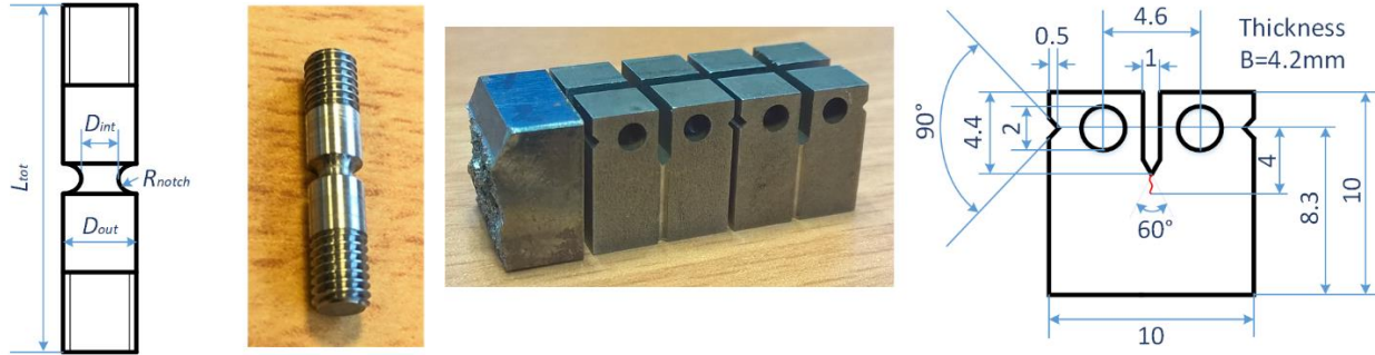
Figure 2 Geometries of round notched tensile specimen and mini-CT specimen
