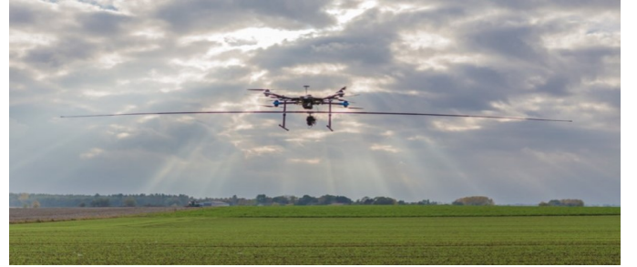
Fig. 3. Prototype drone-borne GPR and drone for soil electrical conductivity mapping.
