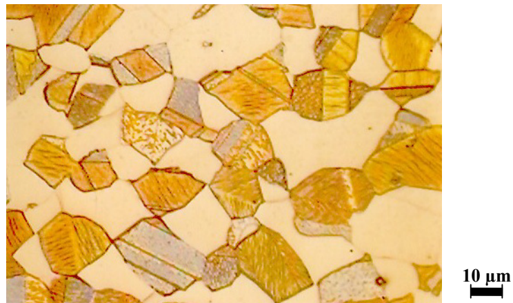
Figure II.1 : Colour etching of steel Mn15.
