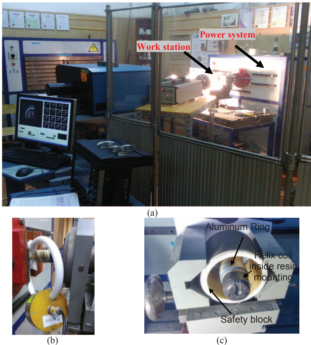
Figure 1: Images showing the of experimental unit and its components (a) overall view of the apparatus, (b) Rogowski coil used for the electric current measurements (c) helix coil and the ring assembly placed inside a large safety block.
