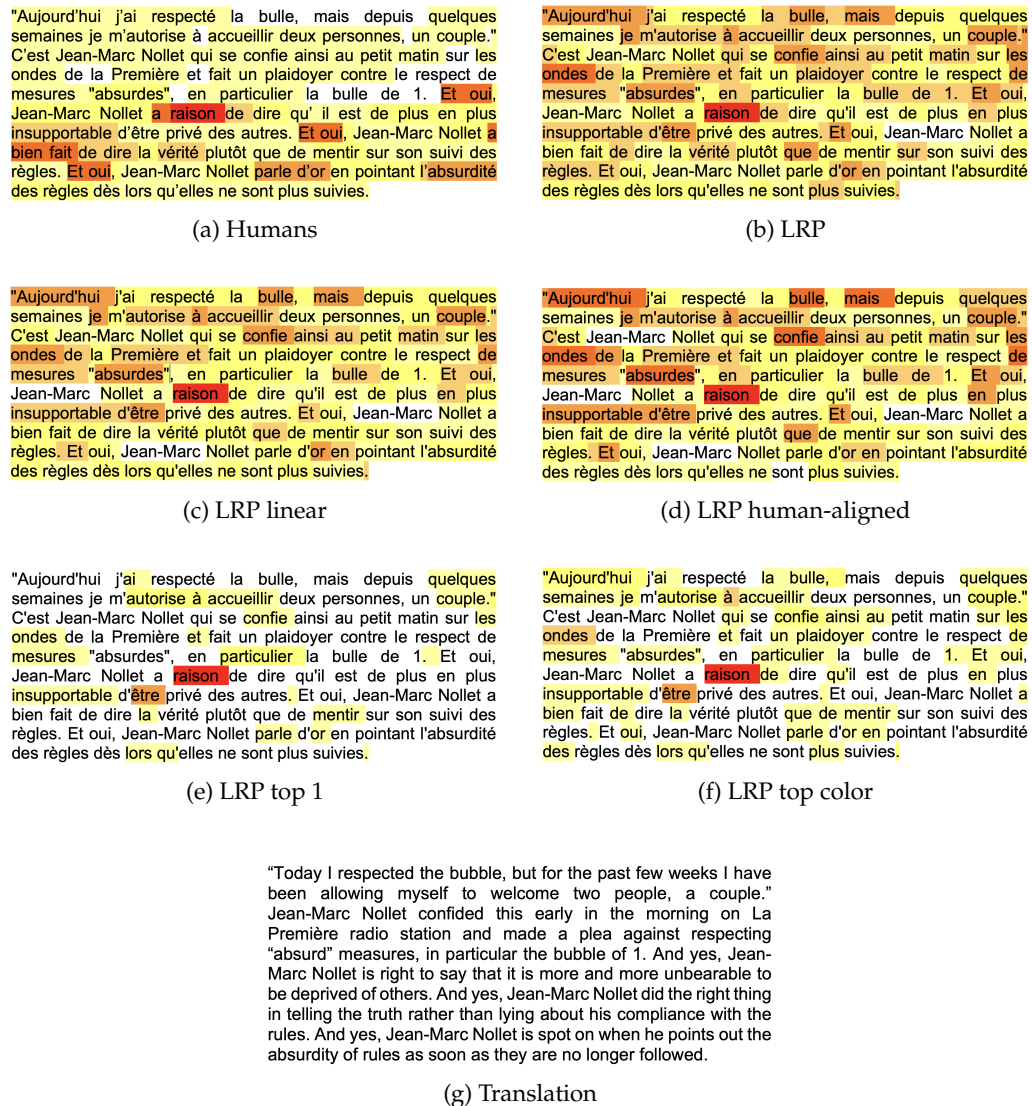
Figure 16: Attention maps of different explanation methods for Opin 2 , an excerpt of an opinion article. For this excerpt, all 42 human annotators agreed on opinion , while 43 out of the 100 equivalent models predicted opinion . Figures (b) to (g) show the aggregations of the explanations provided only by the models who predicted opinion .
