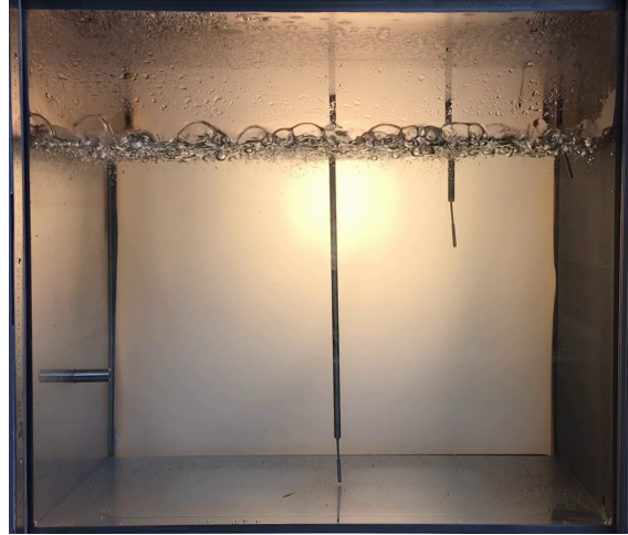
Fig. 6. Overview of the Aquarius pool with a flashing of the superheated water taking place exclusively below the liquid free surface (notice the presence of numerous bubbles at that location).
