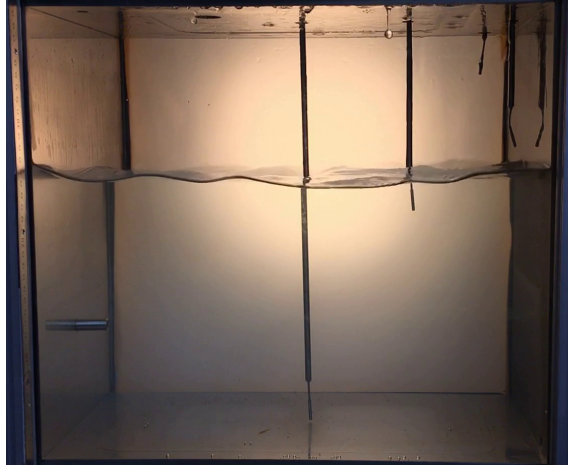
Fig. 7. The late single-phase regime of any gravity-driven pool flashing test conducted by means of the Aquarius device (notice the absence of any bubble). This regime is typically reached when the amount of dissolved oxygen is below an approximate threshold value of 0.7 mg/L.
