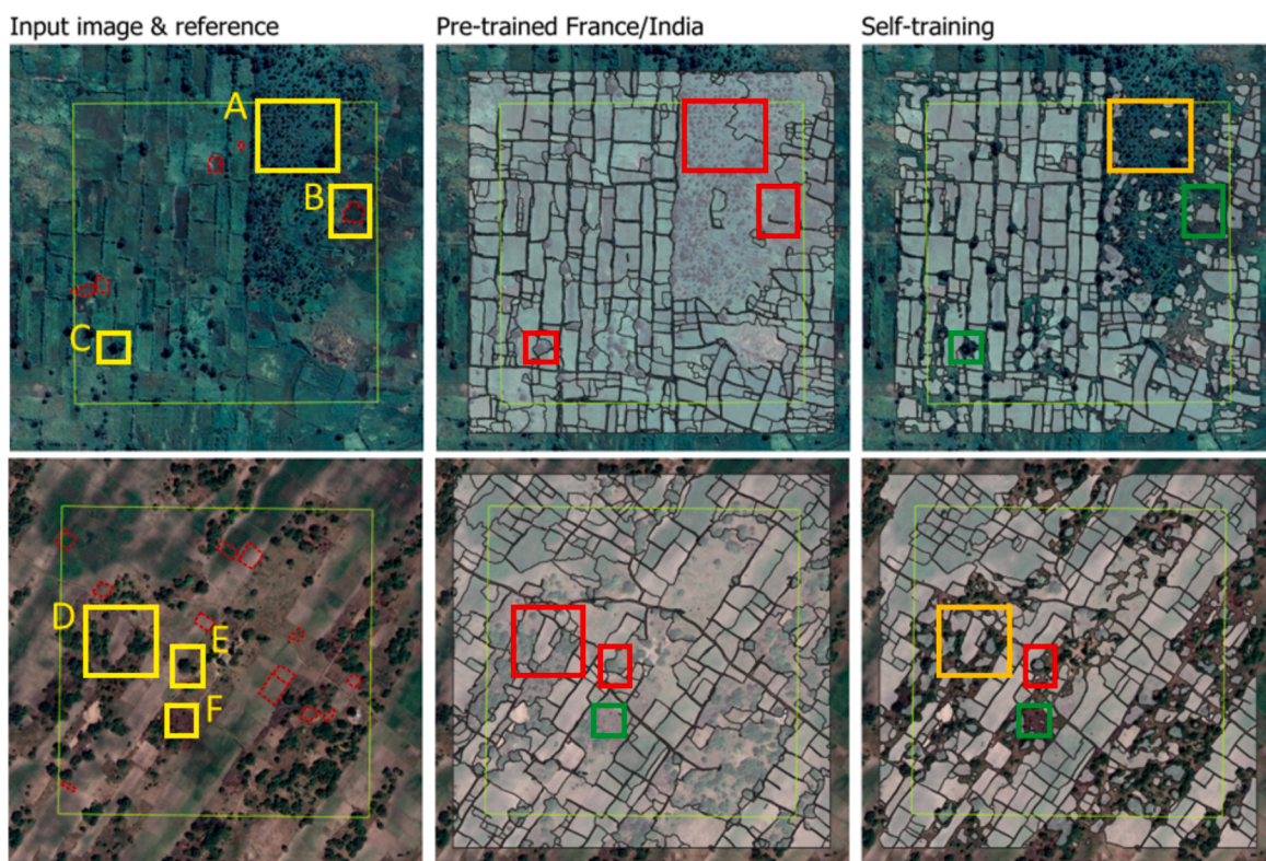
Fig. 13. Example input imagery with human-annotated labels (first column), predictions of the baseline model (second column), and pseudo-labels (third column). Boxes indicate examples of high (green), medium (orange), and low (red) performance of non-cropland identification, relating to the detection of (A) large patches of woody vegetation, (B) isolated fields in non-cropland surroundings, (C) isolated trees, (D) clusters of trees, (E) large trees with irregular canopies, and (F) short-term fallow cropland. (For interpretation of the references to color in this figure legend, the reader is referred to the web version of this article.)
