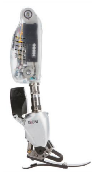
Fig. 9.1: CSEA knee connected to a BiOM ankle prosthesis from the MIT Biomechanics group [80].
