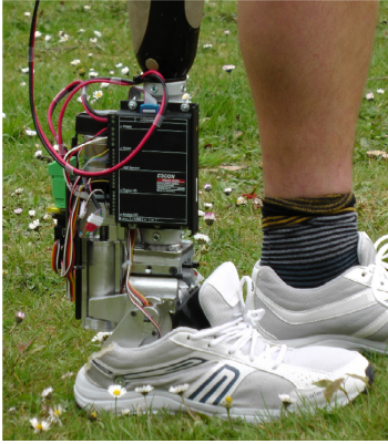
Fig. 2.17: The Ankle Mimicking Prosthetic (AMP-) Foot 3 prototype [17].
