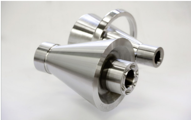
Fig. 6.9: The Cone-Ring-Transmission (KRG) [39].
