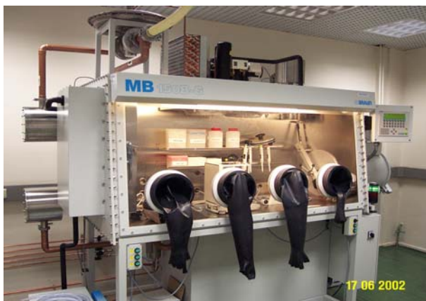
Figure 4.1. Pictures of the glove boxes. a: Jacomex (BS 531 NMT4NMT) glove box, Ar-0.4%CO 2 atmosphere. b: Braun (MB 150B-G) glove box, Ar-5%H 2 -0.4%CO 2 atmosphere.
