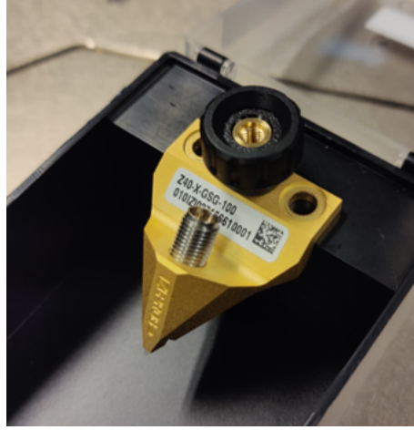
Figure 2.7: |Z| Probe used for high-temperature measurements.
