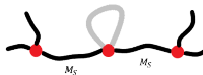
Scheme 3. Elastically Ineffective Loops in the Structure of the Network Caused by Dimerization of Two UPy Units on the Same Polymer Chain
