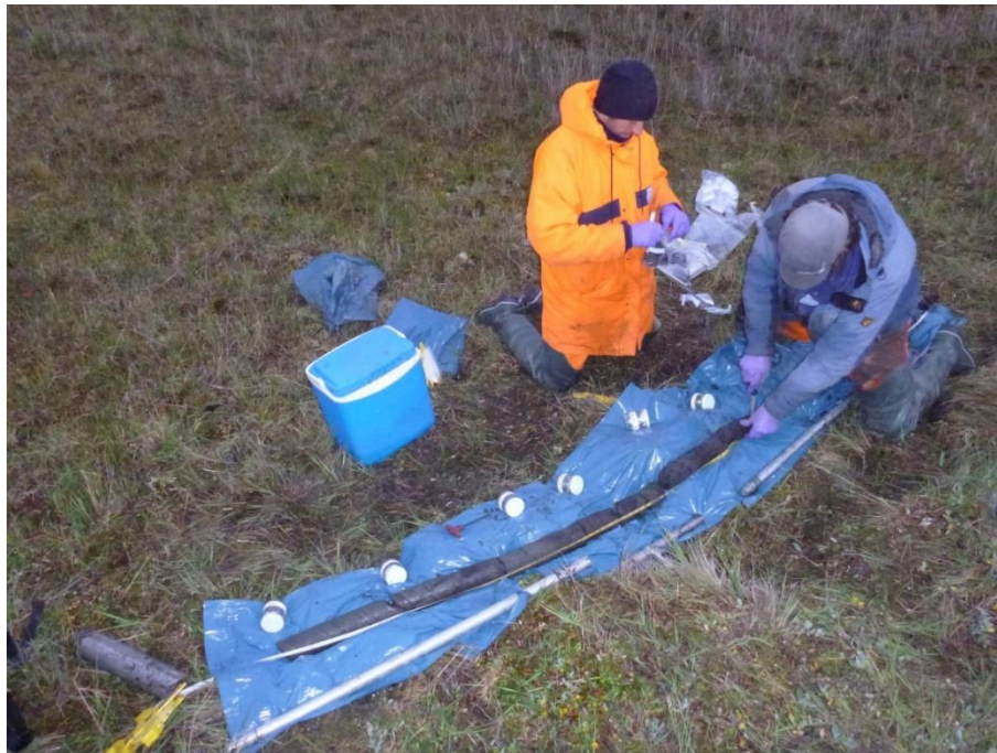
Figure 4.5: Coring technique after SIPRE (Snow, Ice and Permafrost Research Establishment) auger barrel drill and sampling subdivision for a permafrost core in Sobo Sise Island, Siberia (Russia) during 2014 field campaign (photographer: J. Strauss).
