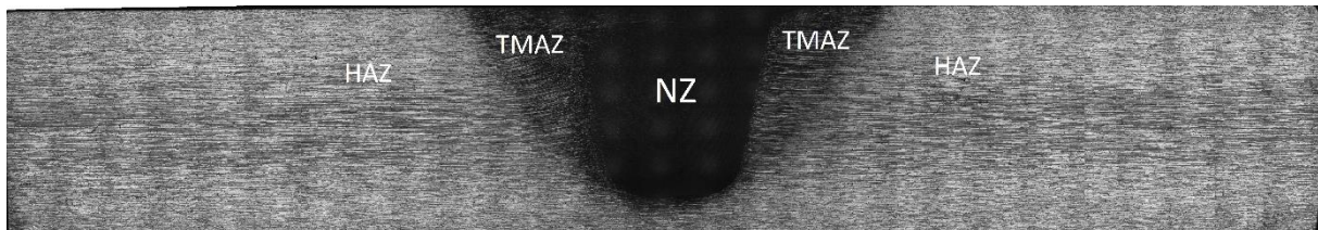
Figure 1: FSPed sample section showing nugget zone (NZ), thermo-mechanically affected zone (TMAZ) and heat affected zone (HAZ)
