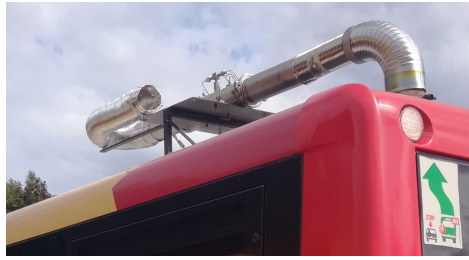
Figure 2. The emissions are measured at the tailpipe of the bus. A sampling probe is installed after the EFM, before guiding the exhaust gases towards the back of the bus.
