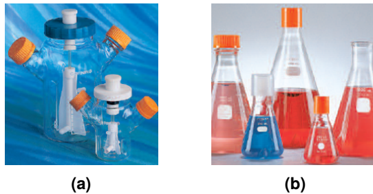
Figure 1.6.: Small-scale dynamic culture systems: (a) spinner flask, (b) shaker flask.[51].
