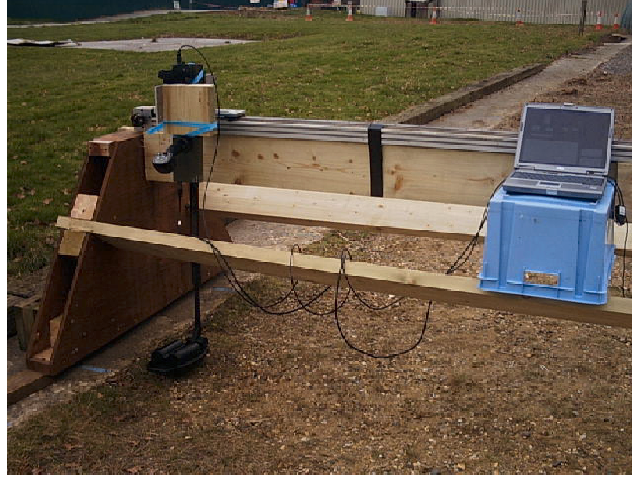
Figure 5.2. Scanning frame with the MINEHOUND unit over the ballast soil.
