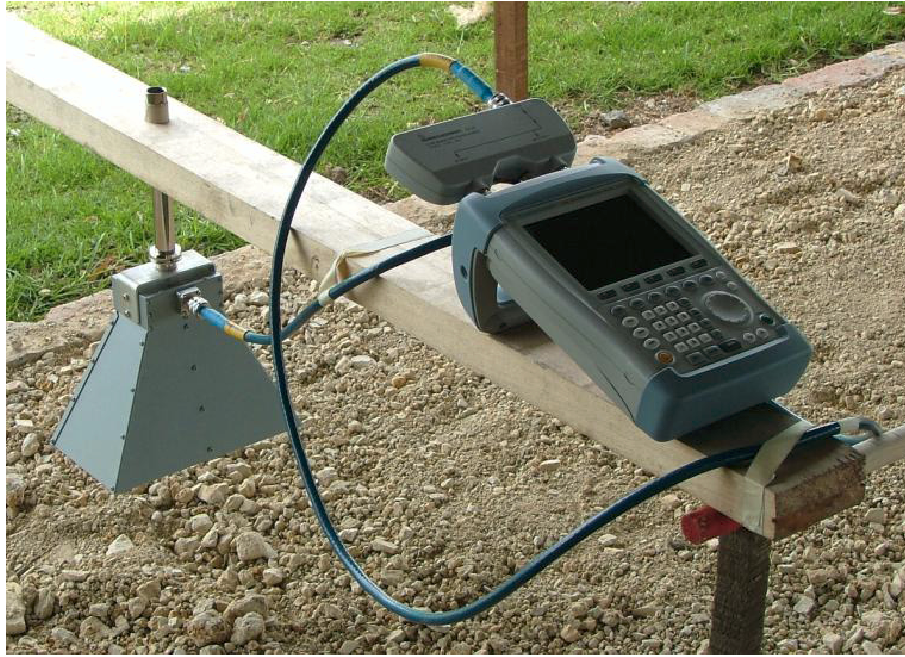
Figure 1.7. The GPR system emulated using the hand-held VNA connected to the horn antenna via a 50-Ohm N-type coaxial cable.
