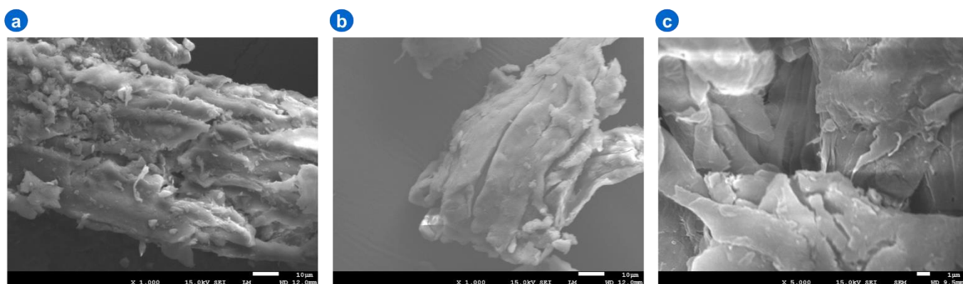
Figure S4 SEM images obtained for untreated birch sawdust (a) and for the solid fraction isolated after treating birch sawdust (3 g, particle size < 2 mm) in a mixture of n-butanol and water (120 mL, 50% v/v), at 200 °C, under 30 bar of N_2 (introduced at ambient temperature), in the presence of Na_2S_2O_4 (1 g), for a duration of 3 hours (b and c). (b) Fiber cells bundles. (c) Detail of fiber cells.
