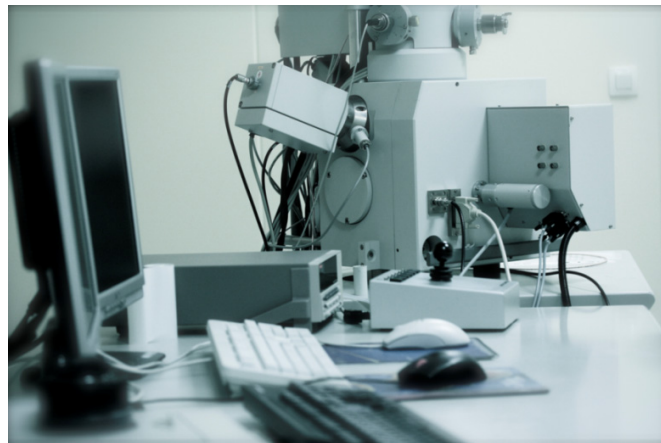
Figure 3.2: Electron lithography system of Philips XL 30S FEG SEM equipped with a RAITH lithography module.
