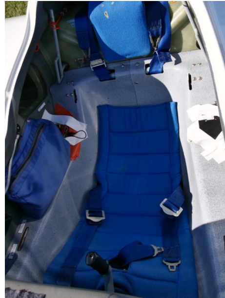
Fig. 2. Mounting of the sensors in the backseat of the glider (FDR-1 on the right, FDR-2 on the left).
