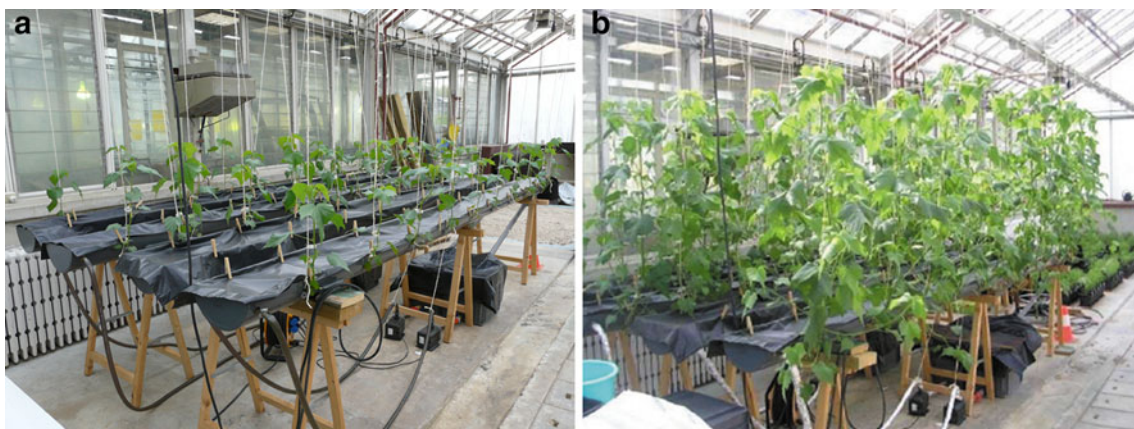
Fig. 1 Experimental device used for NFT culture of Kosteletzkya virginica mature plants. Young seedlings were introduced laterally in a closed gully exhibiting a slope of 1.5 % while a circulating nutrient
