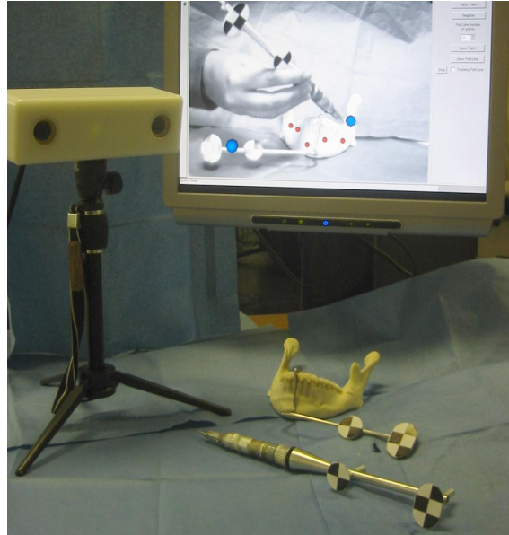
Figure 9.1: System setup - stereo camera and markers attached to the tracked objects.
