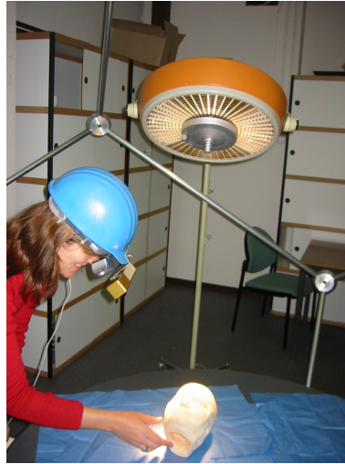
Figure 8.1: Stereo cameras coupled to a 3D stereo glasses and a gypsum phantom representing the patient.
