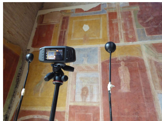
Figure 4. The compact HSI camera during the measurements campaign of the paintings in the main room of the Giove and Ganymede house.
