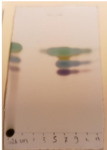
Figure 27: Monitoring the separation of 264 (green-blue, top spot) from 263 (blue, middle spot) and 257 (purple, bottom spot).
